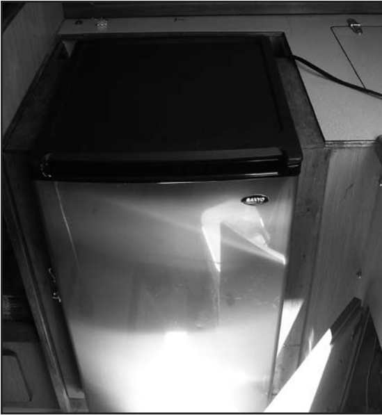
Open this home style refrigerator on starboard tack and one would see the contents all over the cabin sole.
